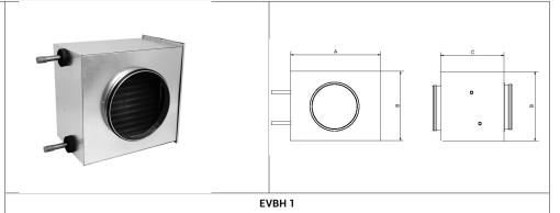
IMPORTANT: The water coil has 125 mm diameter inlet and outlet air flow connections, while the recuperator outlets are 160 mm in diameter. For installation, provide concentric reductions from diameter 160 mm to 125 mm and the corresponding female sleeves.
