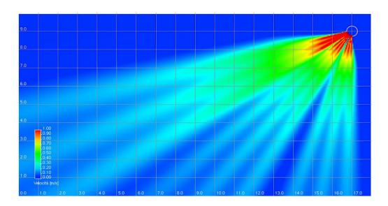
N.B. Diagrams simulated with residual speed 0.2 m at 1800 mm from the ground in a more conservative way than UNI 10339 and UNI EN 13779.
