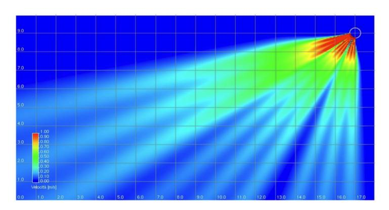
N.B. Diagrams simulated with residual speed 0.2 m at 1800 mm from the ground in a more conservative way than UNI 10339 and UNI EN 13779.
